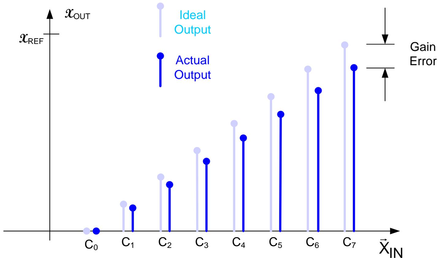
Gain error determined after offset is subtracted from output
