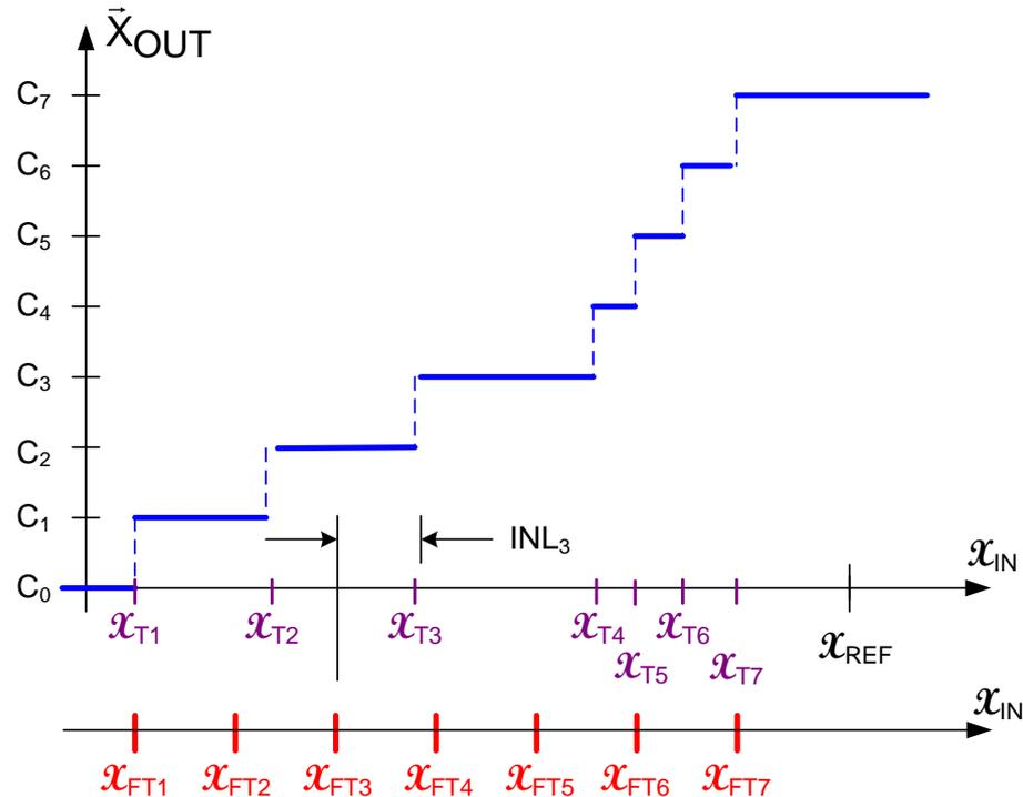
Place  $N-3$  uniformly spaced points between  $X_{T1}$  and  $X_{T(N-1)}$  designated  $X_{FTk}$
