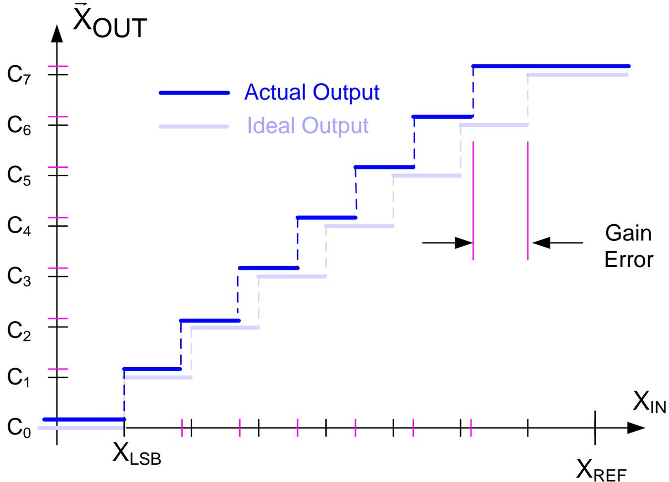
Gain error determined after offset is subtracted from output
