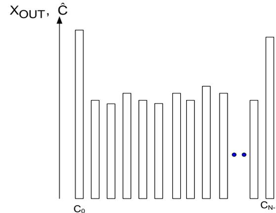
Though INL and DNL for an ADC are rigorously defined, measuring the actual transition points is not practical even if  $n$  is small so code density tests are almost always used to “test” the INL and the DNL
