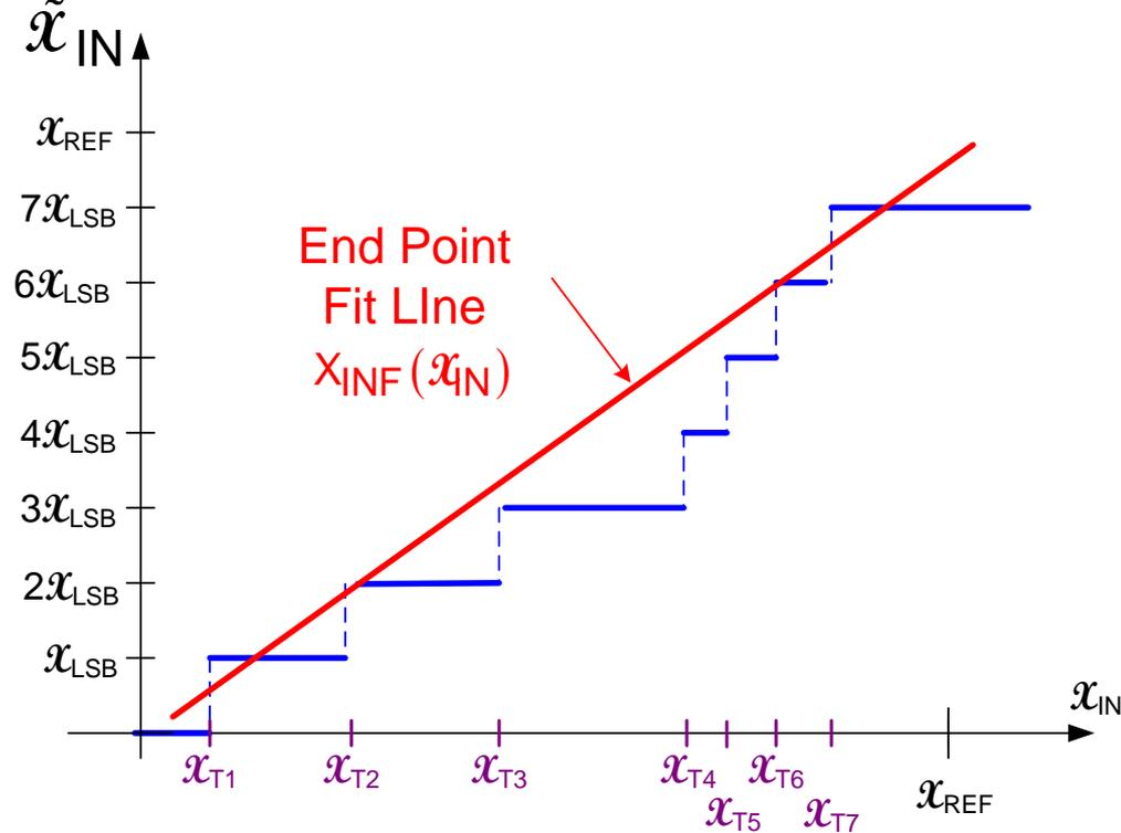
Consider end-point fit line with interpreted output axis
