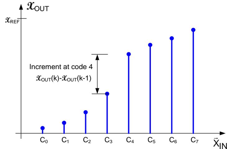
Increment at code  $k$  is a signed quantity and will be negative if  $X_{OUT}(k) < X_{OUT}(k-1)$
