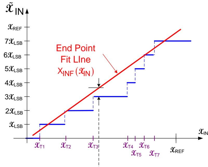
With this definition of INL, the INL of an ideal ADC is  $x_{LSB}/2$  (for  $x_{T1}=x_{LSB}$ )
