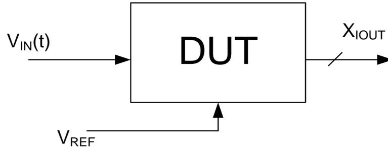
Linearity testing often based upon code density testing
